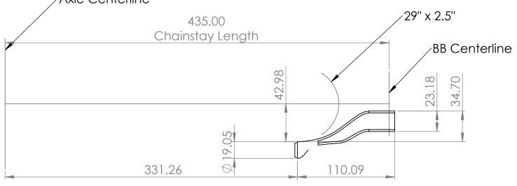
Designed around 1x 36T chainring with boost spacing chainline
